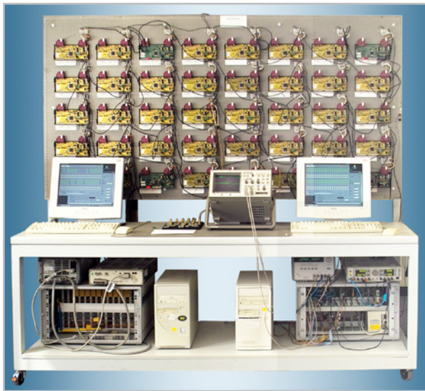
Figure 2b: Transceiver Tester Implementation
