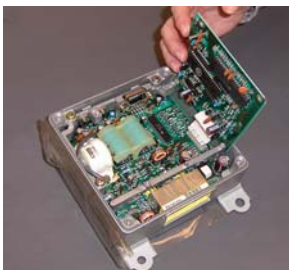
Figure 2: ECM - Example Electronic Control Module
