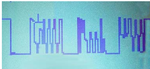
Figure 16: 100 kHz Digital Scope CAN Waveform
