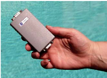
Figure 4: J2534 Pass-Thru Reprogramming Device
