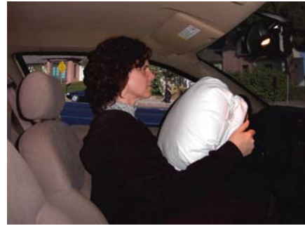
Figure 10 Correct Driver Airbag Deployment
