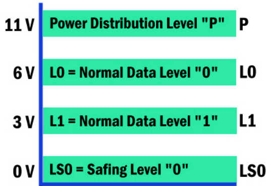
Figure 3 Differential Bus Voltage States
