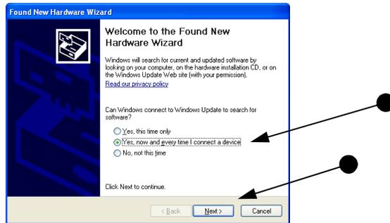
**Step 1:** Connect the VSI-2534 to a power source (Power adapter or powered from the OBD II cable). Note: do not power unit from multiple sources. Power LED must be a solid Green. Connect USB Cable to PC. In some versions of Windows the final step in driver installation is automatic. In others, the Windows Found New Hardware Wizard will run to finalize driver installation. This can take a few moments to come up.
