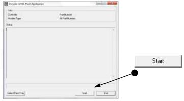
• Make sure the vehicle's Ignition Switch is in the "On" position and then click on the "Start" button. Respond accordingly to the various prompts, such as these shown below.
