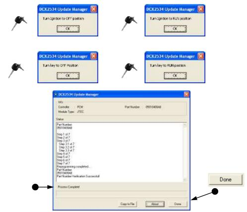
• "Part Number Verification Successful! / Process Complete". Click on "Done" and disconnect tool from vehicle.
