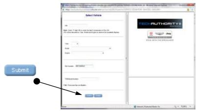
• Identify the vehicle being programmed using one of the available options and click on "Submit". Note: Using the "Part Number" is the best option as it will provide you the only matching update.
