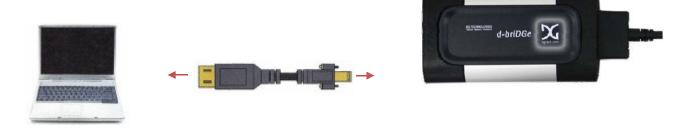
Now, connect the d-briDGe to the vehicle, verifying that the d-briDGe *Power* LED is lit.
