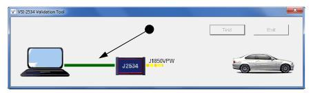
• First, the software will verify proper connection/communication between the PC and the VSI-2534. A solid green bar indicates a proper connection.
