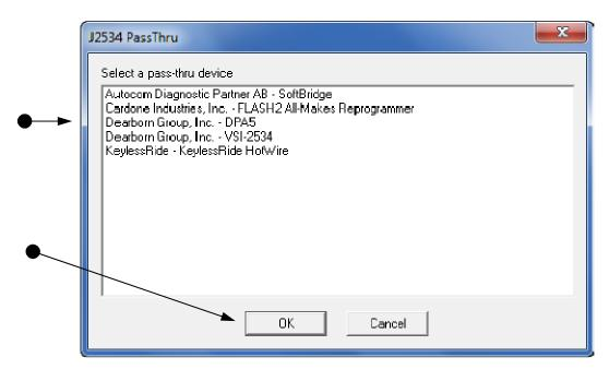
Select the applicable DG J2534 compliant device being used and then "Ok".
