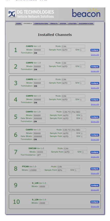
Under the Channels tab is a listing (by channel with version and serial number) of the modules installed on the hardware. It also contains Channel Statistics and driver information.
