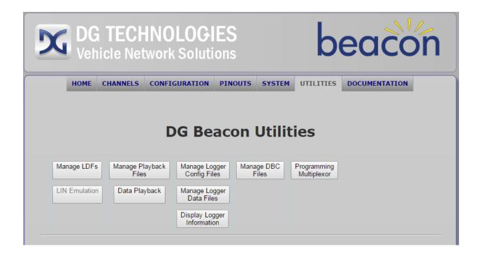
This page provides links to a number of on board utilities, including a utility to manage LIN Definition Files, utilities for use with the built-in data logger program, DBC file management and a programming multiplexor for interfacing to multiple ECUs in an End Of Line or programming environment.
