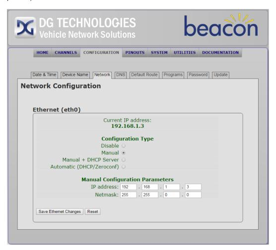
Network configuration – Enter your configuration type (DHCP Client, Static or DHCP Server) and any Static Configuration Parameters, as necessary. To make changes, provide new values where necessary, and click Submit BEACON® Ethernet Changes. Then turn the BEACON® unit off and back on, (i.e., reboot), to invoke the changes. Clicking on Reset will display the previous settings.
