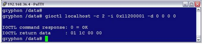
The return data are the BTR values, in this case  $0x01 \ 0x1C \ 0x00 \ 0x00$ . This value corresponds to preset 2 baud rate on the SJA1000 card. Notice that we specified "-d 0 0 0 0" in the gioctol command. This is because, when we get I/O control values, we need to include a data value for each expected returned data value.
