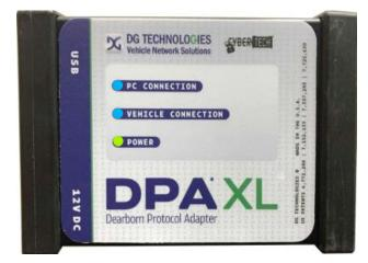
29. Find the DPA XL with the "PC Connection" and "Vehicle Connection" LED's that are blinking blue.
