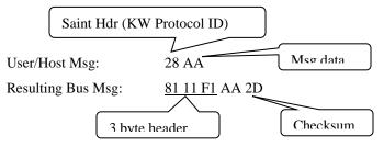
Direct Mode does NOT employ any form of message construction. It is intended to provide users unrestricted control of the message frame content. Message frames are delivered exactly as supplied (unmodified) directly to the bus. The user is responsible for all message frame content including the header and checksum bytes.
