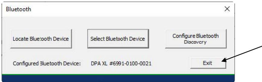
18. Notice the Device ID is now shown at the bottom of the screenshot above. Select [Exit] OR to enable “CyberGuard” so other devices do not recognize the DPA XL device ID, continue below at Step 22.
