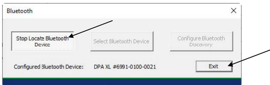
30. Once the PC and Vehicle Connect are found, select [Stop Locate Bluetooth Device], next [Exit], when complete select [OK].
