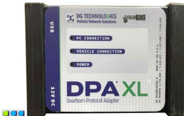
29. Find the DPA XL with the “PC Connection” and “Vehicle Connection” LED’s that are blinking blue.
