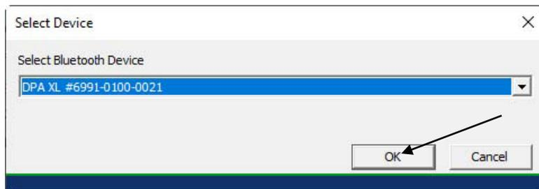
17. From the drop-down menu, choose the “DPA XL #xxxx-xxxx-xxxx” device’, then select [OK]. (Note: Device ID be confirmed by looking at the back of the DPA XL and the bar code number. First 4 digits of the bar code do not apply.)
