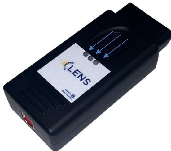
Figure 1 - LENS® LED Indicators
