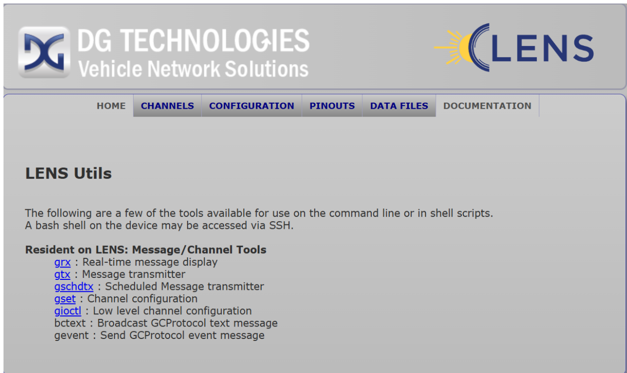
Figure 29 – LENS Utilities Information
